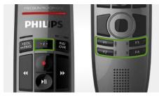
The SpeechMike Premium Touch has freely configurable keys which are especially useful for programming speech recognition commands. The device can be personalized for any user and application.
